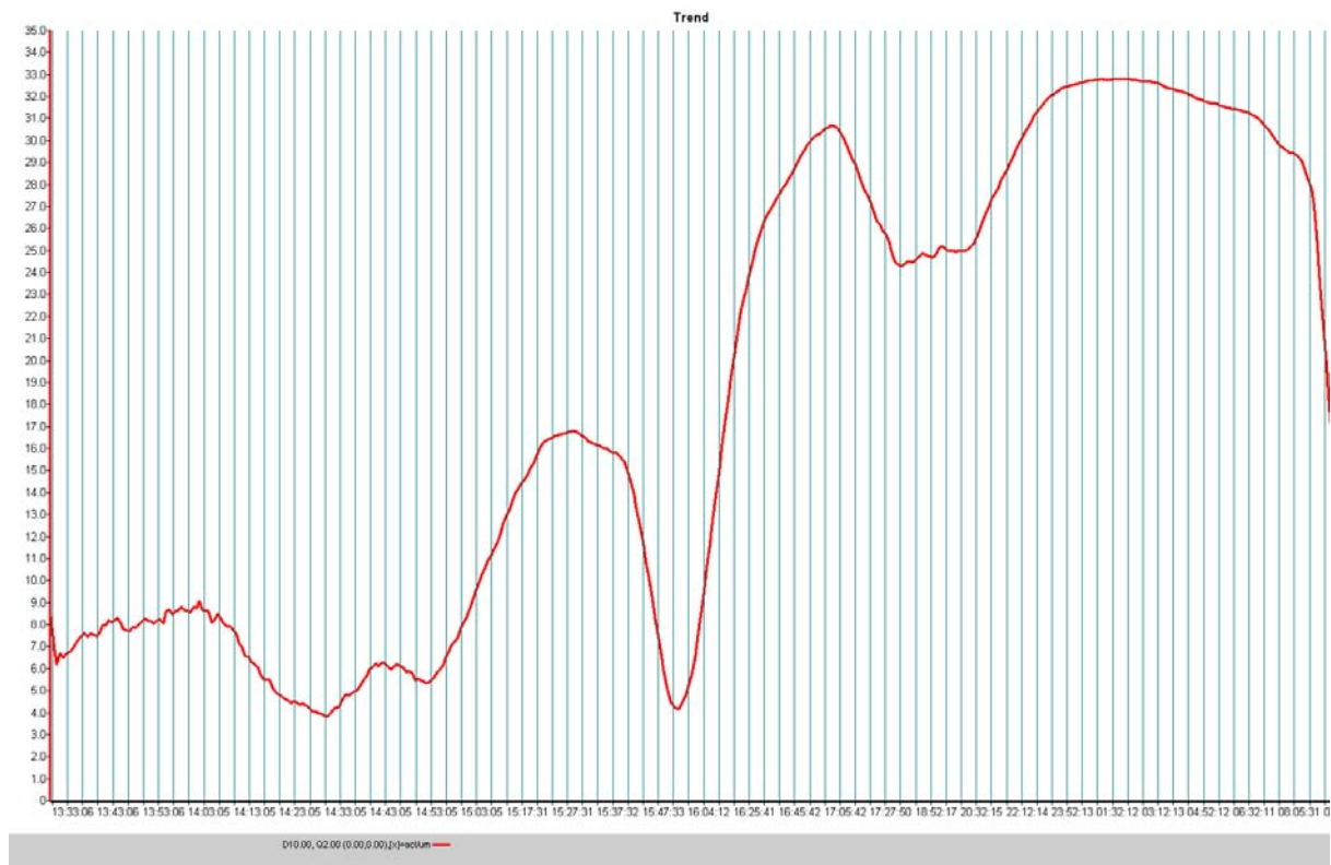
Fig.05 d10/2 over time of total reaction during the polymerisation
